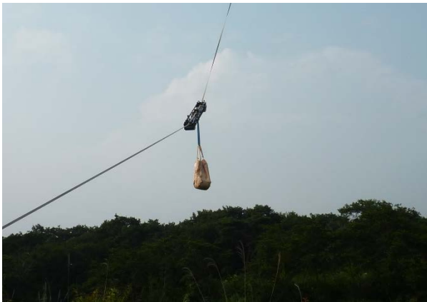
Fig. 5 4th Lab.'s climber with heavy payload
